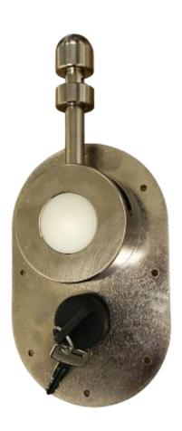
**The Binnacle Mount (+\$295 USD)** is appropriate for boats with wheel steering. It is designed to attach to the 1" grab rail that surrounds most binnacles. It can also attach directly to a binnacle post if no rail is present. It is supplied with longer 20' cables and is ready to install on your binnacle.
