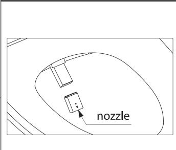
Powered on and not seated: Press the "Nozzle Clean" button on the remote controller, and the washer will automatically extend. If there is dirt in the nozzle orifice, If there is dirt in the nozzle orifice, you can gently hold the washer with one hand and clean it with a toothbrush with the other hand.
