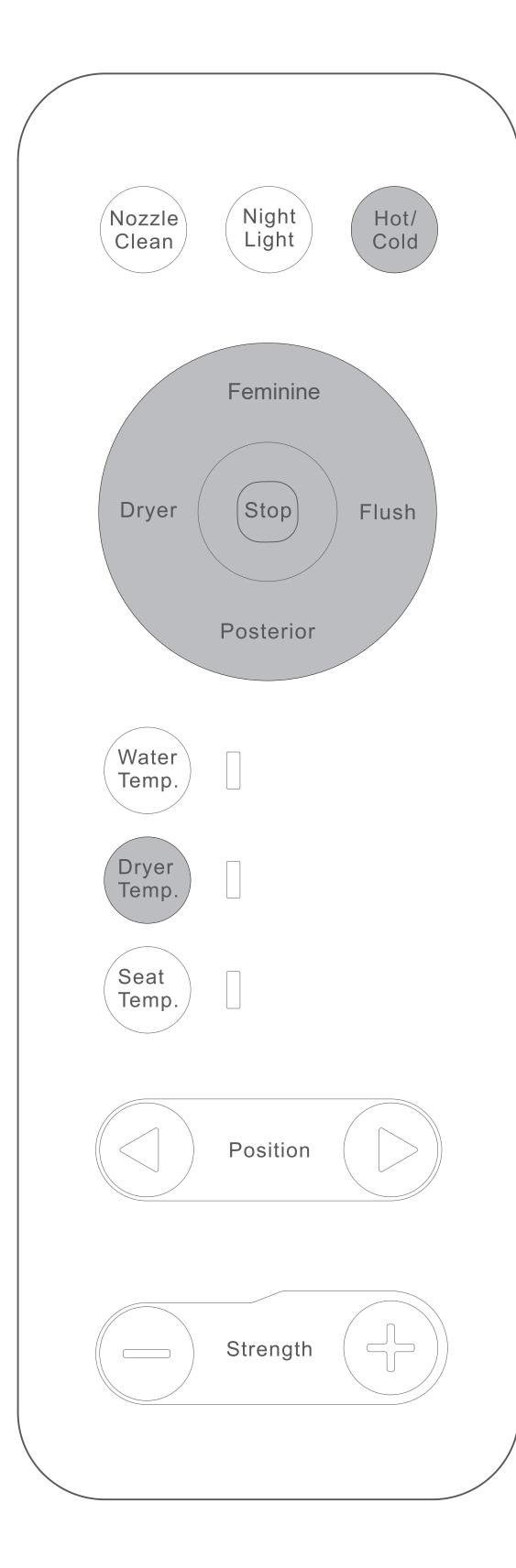
When the key is pressed, display indicator is switched among [Off (display indicator is off)], [Low level (display indicator is in blue)], [Middle level (display indicator is in purple)] and [High level (display indicator is in red)]. Warm air has automatic stop function 4 minutes later.
