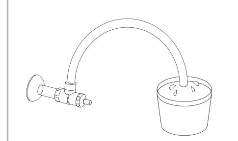
Open the angle valve for water supply. The measured water flow for 10 seconds should exceed 3L.
