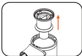
3. Lift the cyclone filter and release it from the cleaner.
