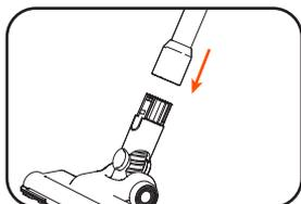
1. Insert the power head into the rod. You will hear a "click" sound when it is securely in place.
