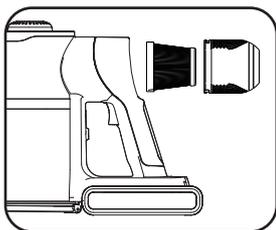
4. To remove the exhaust filter, turn the filter cap anti-clockwise. Then, pull the exhaust filter from the filter cap.
