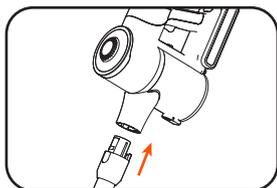
2. To install the rod, insert the plug end of the rod into the air inlet of the cleaner. Once it is securely in place, you will hear a "click" sound.
