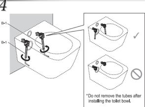
For repairs & maintenance, where the dismantling and reinstalling of the wall hung water closet is concern, it is advisable to change the fixing kit.
