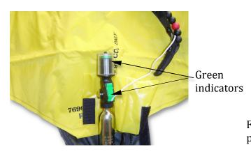
3. Install CO2 cylinder. (½" thread 38 gram 150.6 gram min. wt.) Check for two green indicators.
