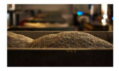
Waste plastics are washed, shredded and pulverised before being placed into a mould to produce a full sheet of EKOply
