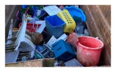
EKOply is produced from 100% mixed waste plastics - mainly PE (Polyethylene) and PP (Polypropylene) which typically ends up being land-filled or incinerated.
