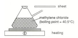
The polishing with methylene chloride vapour should be done in a well ventilated area, if possible underneath an extractor hood. Because of the low boiling point of methylene chloride, it has to be heated only slightly to create vapour.
