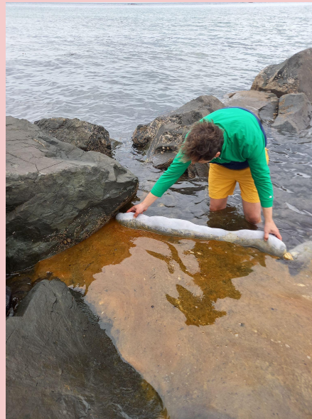
Fry Taylor using hair booms to contain an oil spill in Ireland.
