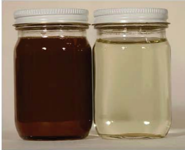
Figure 5. Fouled extrusion system distilled water coolant (left) and one maintained with EPF (right).
