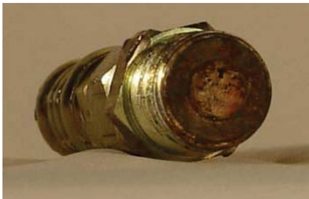
Figure 2. Plugged extruder 3/8 inch zone inlet coupling.
