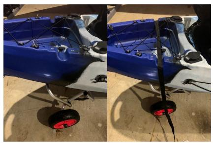
When using your kayak trolley we recommend putting it under your kayak as above. Then weave the securing strap through the trolling motor mount recess as so.
