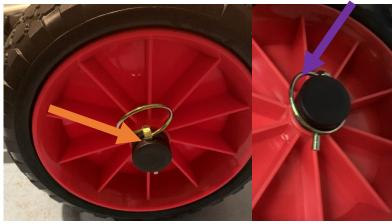
Push the locking pin through the aligned holes (orange arrow) and flip the ring over so it locks the pin in place (purple arrow). Now you've completed one wheel, repeat the actions for the second wheel.
