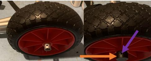
Your kayak trolley should come disassembled as per the above. With the main frame, 2 x wheels, 2 x black locking nuts, 2 x locking pins and 1 x kayak strap. First put one wheel one of the ends. Next put the black wheel cap on (orange arrow) and align the holes (purple arrow).
