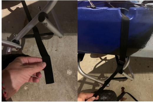
Run the strap through the lower arm section and cinch it through the buckle and tighten.
