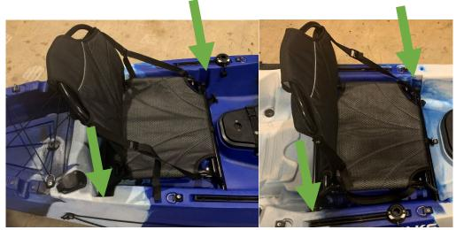
Insert the forward and back seats as per the above. There are specific slots for each of the seats to secure them from moving around during paddling.
