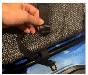
At the front of each seat is a security strap to secure your seat from being lost should you tip your kayak over when on the water.
