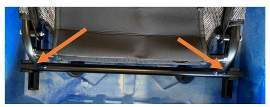
Lastly connect and secure the two side straps which hold the back of the seat upwards. Secure this in a slightly off of 90 degree upright position, this can be further adjusted once you're on the water.
