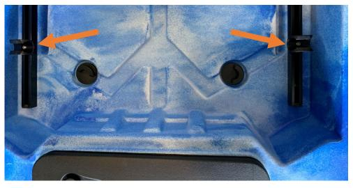
Sit the back bar of the seat on top of the brackets, but don't pop them in yet. Screw the front of the seat into the two front slider receivers.
