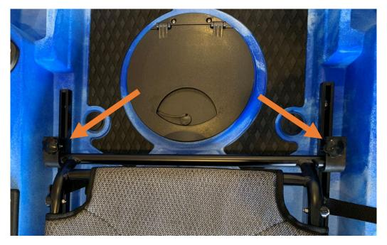
And then push the back bar down into the back seat brackets to secure that.
