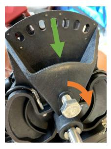
Once the pedals have been inserted into the drive unit, then drop the pedal drive into place, and the kayak locking pins should lock over the pins.
