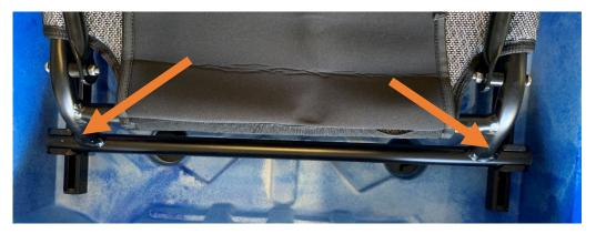
Lastly connect and secure the two side straps which hold the back of the seat upwards. Secure this in a slightly off of 90 degree upright position, this can be further adjusted once you're on the water. Also remember to take your allen wrench on your first couple of outings in case you want to further adjust your seat location.
