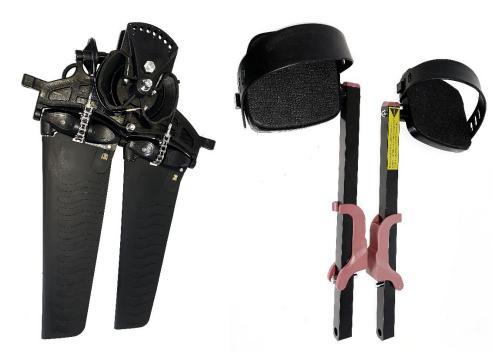
Note the numbering on the top of the pedal drive unit, to know which is forward, '1' will be at the bottom (closest to the seat). For the time being don't worry about the numbering as this will help you set the correct leg length later on. Insert each pedal (green arrow) with the main bolt fully un-screwed (orange arrow), and while holding the red handle depressed. Aim
