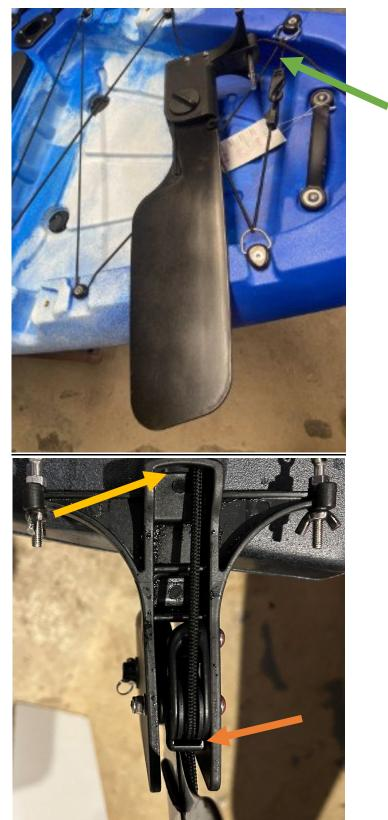
Next, you'll you to thread it through the two holes in the actual rudder blade. Note the blade below is in the up position. Thread the line first through the hole that is near the curve of the rudder blade (Green Arrow, it will be the hole right at the back of the kayak if the
