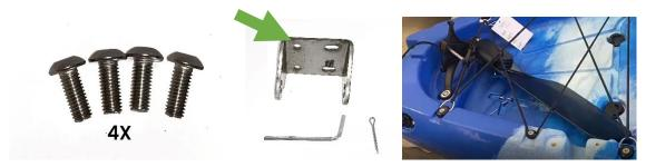
Place the two holes (green arrow) of the bracket at the top when securing the bracket to the back of the kayak. And insert the 4 screws with the allen wrench.
