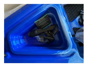
The rudder will already be strung (for putting in our pulling out of the water) and ready for use and secured in the rear hatch behind the seat and underneath the internal basket.
