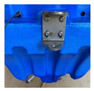
Next, ensure your rudder is untangled and the lines run free. Put the pin of the rudder through the rudder bracket holes. Check that the raising and lowering of the rudder operates smoothly. Next put in the rudder security pin through the hole at the bottom of the rudder pin. Using a knife, screwdriver or pliers open the security pin ends (green arrow) to prevent losing the rudder, through the pin popping out.
