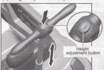
Press the top button of the push handle for unlocking to shorten or lengthen the push handle, and lock the push handle to another height when hearing the "click" sound.
