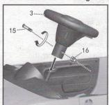
(Mount the battery of the steering wheel as per Point 4.) Install the steering wheel (part 3) on the J-shaped stick, and then tighten it with the steering wheel screw (part 15) and locknut (part 16).
