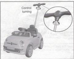
While pushing the baby car, swing the push handle from side to side to realize the synchronous rotation of the push handle and front-wheel.
