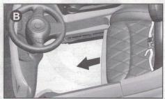
Push the foot treadle according to the arrow direction in Figure (a) to draw back the foot treadle to the seat bottom, conversely, pull the foot treadle according to the arrow direction in Figure (b) to pull out the foot treadle from the seat bottom.
