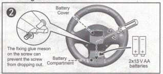
Battery box is at the bottom of the steering wheel. Turn over the steering wheel and open the cover of the battery box. To replace the batteries, firstly take out old batteries, align positive and negative poles of the battery, install two AA batteries, close the cover and tighten the screws.
