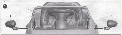
Install the windshield (part 2) and rear-view mirror (part 4) at the assigned location of the car front end, find each buckle position before installation, and then press it forcefully until each buckle position is tight.
