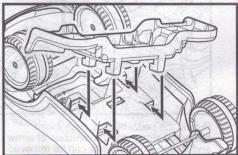
Insert the pedal buckles into the assigned location of the car bottom and push them forward along with the direction of arrow until fasten them.
