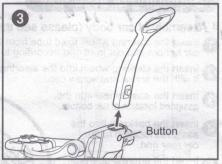
Press the button under the push knob, the push knob can be removed.
