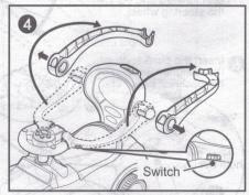
Push the switch of the armrest guardrail and spin it backward, the armrest guardrail can be removed.
