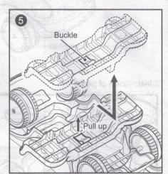
Pull up the pedal buckle, push them backward along with the direction of arrow and lift upward, the pedal can be removed.
