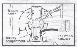
Open the steering wheel battery cover, find the positive pole and negative pole, and put 2AA batteries into the compartment properly, then close the battery cover and fix it with the screw (as shown in the Figure).
