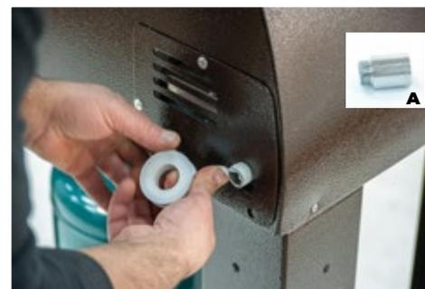
**1.** Insulate the oven gas connection with Teflon tape (A) and screw in the gas hose.
