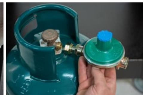
**2.** Screw the gas regulator into the bottle valve and turn the bolt counterclockwise. Use the gas bottle spanner to tighten and not to damage the gasket and the watertight seal.
