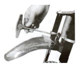
Install plate, put a spacer ring first, then fix it. And insert fender to plate.
