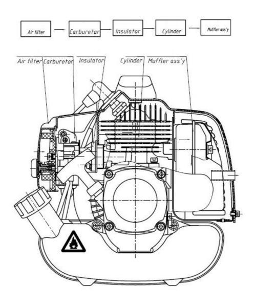
The exhaust gas is discharged after the second combustion of the catalyst.
