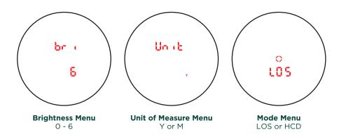
Once you have the desired settings, press and hold the **MODE** button for 3 seconds until you see the power on screen again. At this point the rangefinder is ready for scanning objects.
