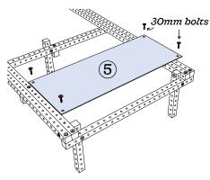
Attach panel 5 to the 3rd hole of inner long rail using the 30mm bolts. Repeat for panel 3 and 1.
