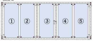
For panel 2 and 4 you will need to loosen the 60mm bolt used to attach the rail and pass it through the panel. Use the 30mm bolt for the other two holes.
