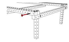
Use the 90mm bolt to secure the short rail to the two long rails.
