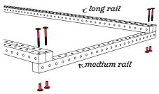
Attach using the 60mm bolts.\*
