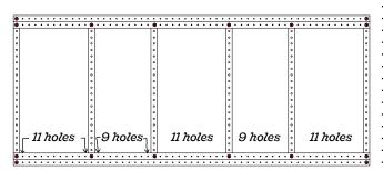
Attach the remaining medium rails to the inner long rail, counting the holes to determine the spacing between each rail.
