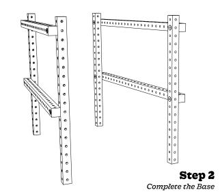
Attach short rail to inside of the medium rail, overlapping all 3 rails to create a tri-joint. Repeat for second shelf and on other side.
