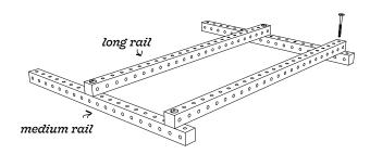
Attach the long rail to the medium rail according to desired shelf height.\* Repeat so you have a set of two legs.
