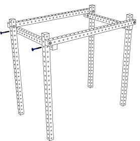
Attach medium rail to short rail, overlapping all 3 rails to create a tri-joint.
