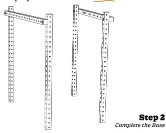
Attach the 20" (short) rail to inside of medium rail. Repeat on other side of table.
