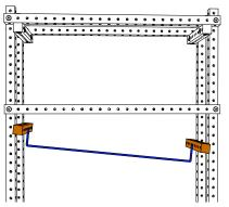
The hanging rod is sandwiched between the two remaining short rails before attaching to the rack.
