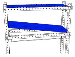
Slide in shelves, loosening bolts if they don't easily slip in. Shelves are reversible and can be installed as a tray or surface.
