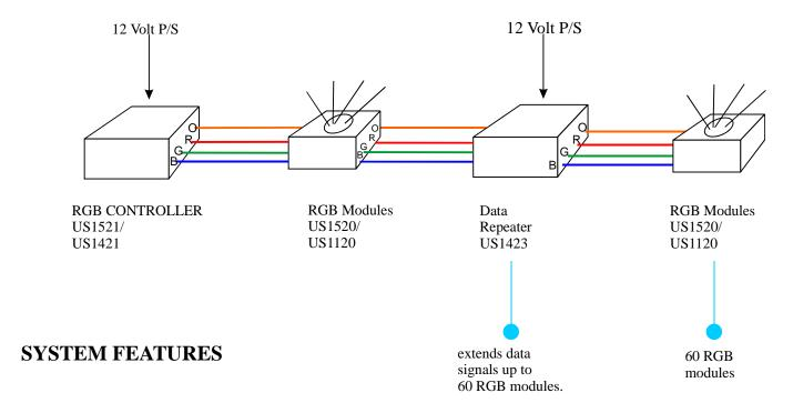
RGB controller US1421/ US1521 controls up to 60 RGB modules. A data repeater is added to extend the data signal to another 60 RGB modules.
