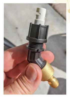
At the low setting, the sprayer output is 40 PSI. At 40 PSI, the white Floodjet tip will allow .8 gallons per minute (GPM) of liquid to flow. At that flow rate, the entire 4 gallon sprayer can be emptied in 5 minutes. (4/.8 = 5)
