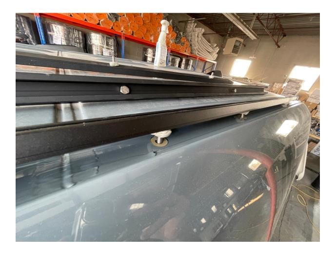
4. Install the washer and tighten the self locking nuts included in the package on the inside if the van.
