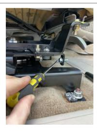
3. Once the bolt is through the hole – thread on the plastic handle until it completely seats.
