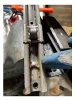
6. Place the inner part of the seat track into the outer (black) part of the seat track. You must ensure the front wheel/bearing assembly does not come forward of the detent in the inner part of the seat track indicated in the previous step.
