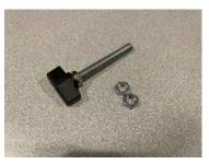
2. Flip over the swivel assembly and place the threaded lock handle (#3) through the outermost hole on the lock arm and thread on the two 3/8-16 jam nuts (#4)
