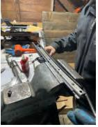
7. Using a hammer and punch – softly drive the inner seat rail back into the outer (black) part of the seat track
