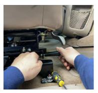
4. Using a wrench on the bolt and holding the handle with you hand – tighten the bolt until it is good and tight. Don't overdo it – the handle threads are brass and will strip if you put too much "oomph" into this step.
