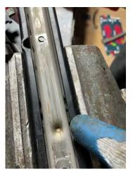
9. Re-attach the locking detent spring. Verify the locking detent snaps into place as you move the slider into a locking position.
