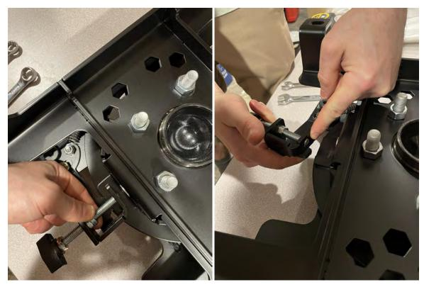
4. Grab two 9/16 wrenches. With the jam nuts (#4) in the correct position, use one wrench to hold the outermost (i.e. the one furthest from the center of the swivel) jam nut stationary and use the second wrench to turn the innermost jam nut *counter clockwise* to lock or "jam" the nuts together.
