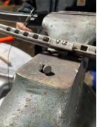
4. Now onto re-assembly. Ensure the rear most roller wheel/bearing assembly is behind the round protrusion on the outer (black) seat track.
