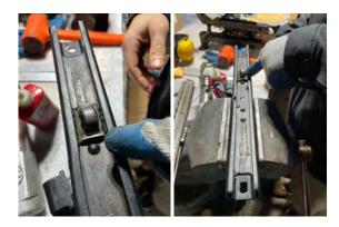
5. Ensure the front roller is behind the protrusion on the inner part of the seat track, as pictured below:
