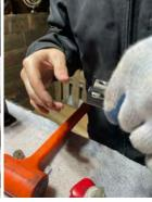
2. Using a hammer and punch (I used a 3" bolt), drive the inner seat rail forward until it releases from the outer (black) portion of the seat track. Remove the inner portion of the seat track.
