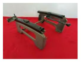
4. Disconnect the two parts of the seat pedestal by removing the center support bolts and unhooking the adjustment lever cable.
