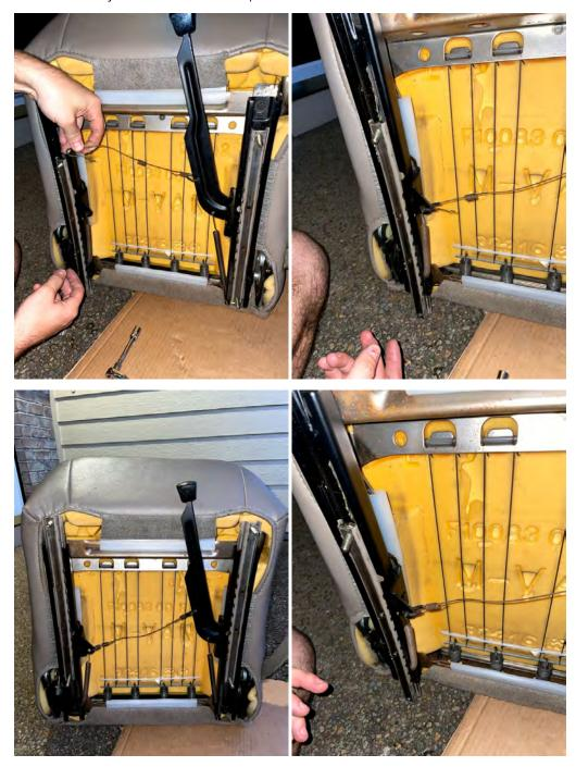
4. Place the seat base/tracks onto the swivel base matching each 5/16" bolt with its corresponding slot on the swivel base. This may involve some cussing – but it will fit.
