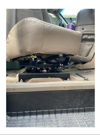
WARNING: While the vehicle is in motion, the seat MUST be in the forward facing position with the threaded lock securely engaged.
