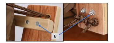
6. Insert a hex bolt (front to back) into each hole and tighten nut and washer using the wrench included in the kit. Tighten each bolt until it is flush with the front side of the wood.
