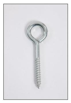
Locate the ceiling beam/joist by using a stud finder or tapping and verifying with a small nail. Be sure to locate the exact center of the ceiling joist for the most secure installation. Using a 3/16" (3mm) wood drill bit, drill a starter hole (approx. 4" or 10 cm deep) perpendicular to the ceiling. Screw in the supplied eye bolts until all threads have disappeared into the joist. Do not loosen or adjust once in place.
