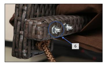
6. Insert a hex bolt (front to back) into each hole and tighten nut and washer using the wrench included in the kit. Tighten each bolt until it is flush with the front side of the wicker.
