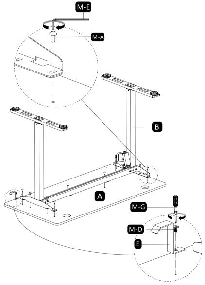
2. Attach Hook (E) to Tabletop (A). Use Screw (M-D) and Screwdriver (M-G) to tighten them.
