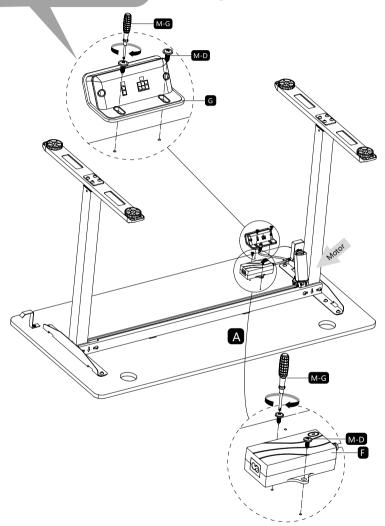
2. Align Power Adapter (F) with the pilot holes, and then tighten it with Screw (M-D) and Screwdriver (M-G).
