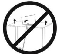
Leave enough slack in cables to allow for full range of vertical motion.
