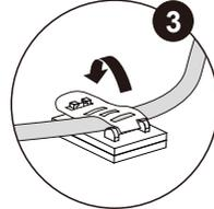
3 Fasten cables with the cable clips.
