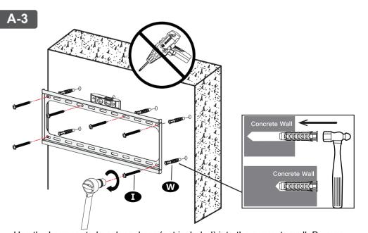
Use the hammer to knock anchors (not included) into the concrete wall. Be sure the anchors are seated flush with the concrete surface.
