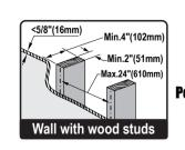
**CAUTION:** Avoid potential personal injuries and property damage! Drywall covering the wall must not exceed 5/8 in. (16 mm). Minimum wood stud size: nominal 2 x 4 in. (51 x 102 mm) actual 1 ½ x 3 ½ in. (38 x 89 mm).
