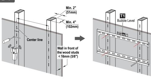
Locate your studs. Verify and mark the center of the stud by finding the stud edges using awl and stud finder. Line up the holes with your stud center line. Level the wall plate and mark the pilot hole locations.
