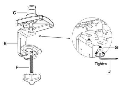
Secure stand to the desktop by tightening clamp (F).
