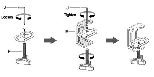
Mount clamp (E) to the bottom of base (C) by tightening bolts (G) with 4mm Allen
