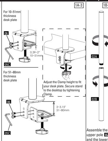
Secure the clamp bracket to the L plate with the
