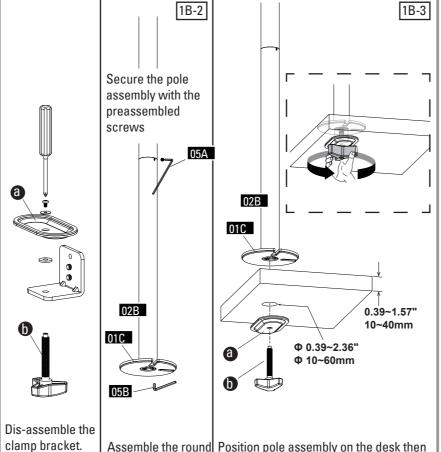
the marked parts plate **01C** to the and will be lower pole 02B used in next step. with the preassembled screws.
