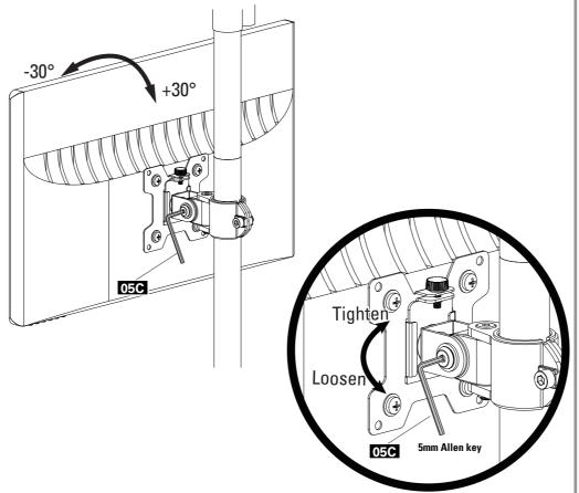
Loosen tilting bolts, pull monitor to your desired angle, then fasten tilting bolts with the 5mm Allen key 05C.
