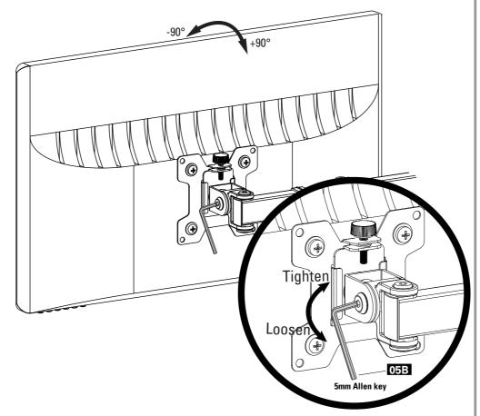
Loosen tilting bolts, pull monitor to your desired angle, then fasten tilting bolts with the 5mm Allen key 05B.
