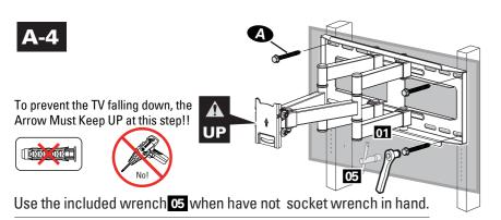
Install wall plate 01 using lag bolts A with Socket Wrench, NO Electrodrill. Tighten the lag bolts A until they are pulled firmly against the wall plate 01.
