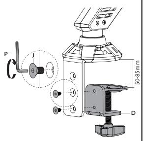
Attach bracket cover (E)to bracket(C). Tighten the clamp to the desktop using the plastic knob or by using 6mm allen key (R).
