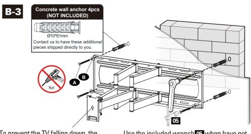
To prevent the TV falling down, the Arrow Must Keep UP at this step!!
