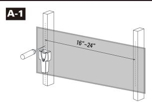
Locate your studs. Verify and mark the center of the studs by finding the stud edges using an awl, a thin nail, and an edge-to-edge stud finder.
