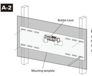
Position the mounting template at your desired height and line up the holes with your stud center line. Level the mounting template and mark the pilot hole locations.
