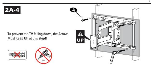
Install wall plate of using lag bolts A with Socket Wrench, NO Electrodrill. Tighten the lag bolts A until they are pulled firmly against the wall plate 01
