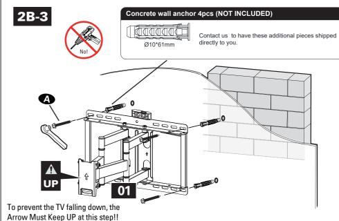
Install wall plate 01 using lag bolts A and anchor (not included). Tighten the lag bolts (A) until they are pulled firmly against the wall plate 01.
