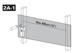
Locate your studs. Verify and mark the center of the studs by finding the stud edges using an awl, a thin nail, and an edge-to-edge stud finder.
