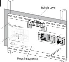
Position the mounting template at your desired height and line up the holes with your stud center line. Level the mounting template and mark the pilot hole locations.
