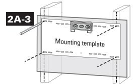
Position the mounting template at your desired height and line up the holes with your stud center line. Level the mounting template and mark the pilot hole locations.
