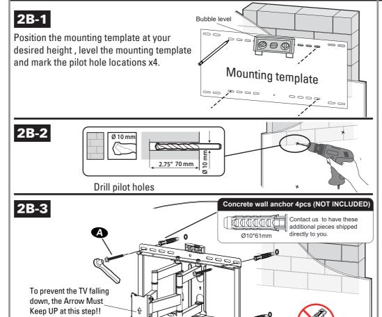
Install wall plate 01 using lag bolts (A) and anchor (not included).
