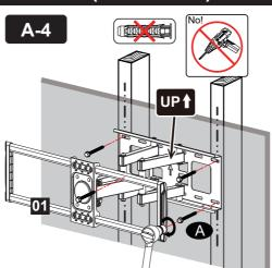
Install wall plate using lag bolts and washer with Socket Wrench, NO Electrodrill.
