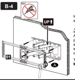
Install wall plate using lag bolts, washer and anchor with Socket Wrench, NO Electrodrill.
