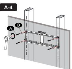
**A** CAUTION: To avoid potential personal injury or property damage: All 4 lag bolts A MUST BE firmly tightened to prevent unwanted movement of the wall
