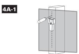
Locate your studs. Verify and mark the center of the stud by finding the stud edges using an awl, a thin nail, or an edge-to-edge stud finder.
