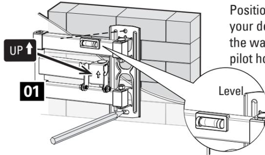
Position the wall plate **01** at your desired height, level the wall plate and mark the pilot hole locations x2.
