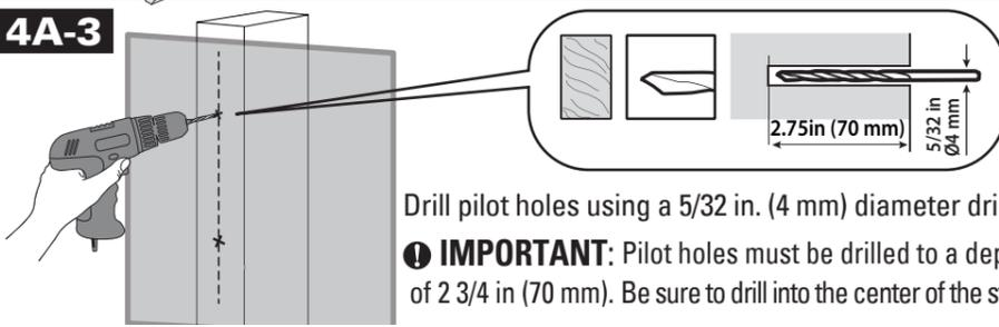
Drill pilot holes using a 5/32 in. (4 mm) diameter drill bit.
