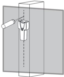
Locate your studs. Verify and mark the center of the stud by finding the stud edges using an awl, a thin nail, or an edge-to-edge stud finder.
