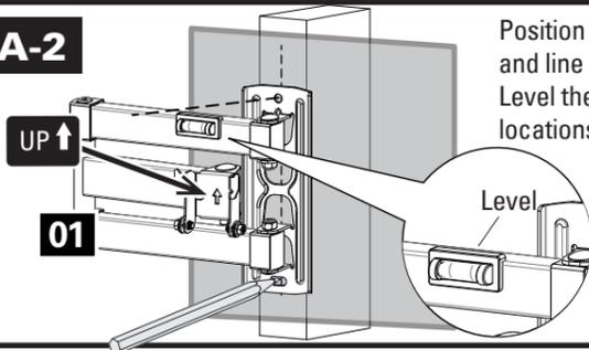
Position the wall plate **01** at your desired height and line up the holes with your stud center line. Level the wall plate and mark the pilot hole locations x2.
