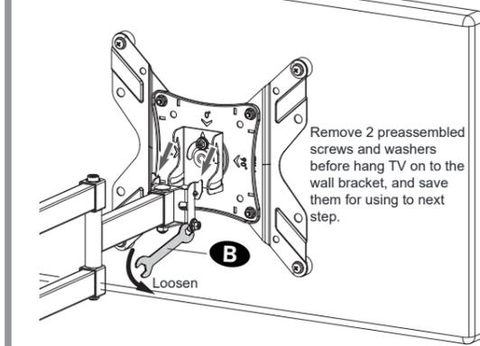
Remove 2 preassembled screws and washers before hang TV on to the wall bracket, and save them for using to next step.
