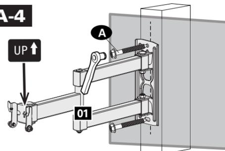
Install wall plate **01** using lag bolts **A** with **Socket Wrench, NO Electrodrill**. Tighten the lag bolts **A** until they are pulled firmly against the wall plate **01**.
