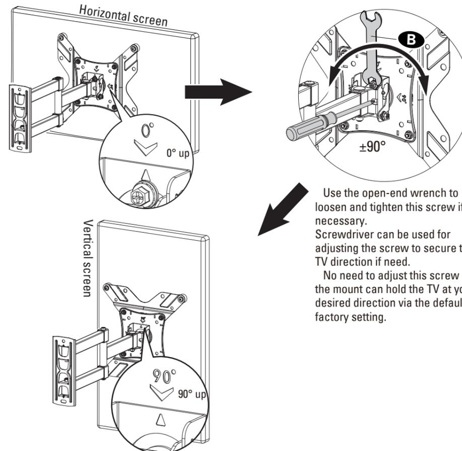
Use the open-end wrench to loosen and tighten this screw if necessary. Screwdriver can be used for adjusting the screw to secure the TV direction if need. No need to adjust this screw if the mount can hold the TV at your desired direction via the default factory setting.
