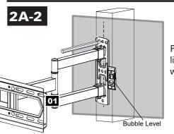
Position the wall plate 01 at your desired height and line up the holes with your stud center line. Level the wall plate and mark the pilot hole locations.
