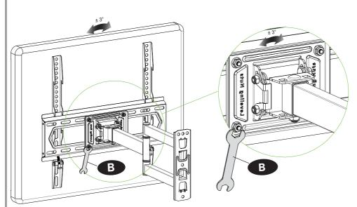
If needed, TV can be leveled ±3 degrees via adjusting the 4 nuts with the open-end wrench.
