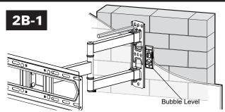
Position the wall plate 01 at your desired height, level the wall plate and mark the pilot hole locations x3.
