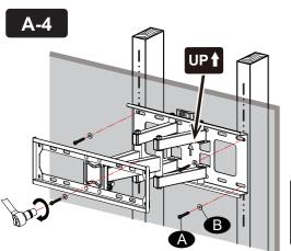
Ensure the lag bolts to be screwed into the studs tightly and securely.
