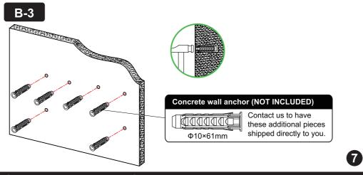
**OPTION B: Solid Concrete or Brick Wall Installation**
