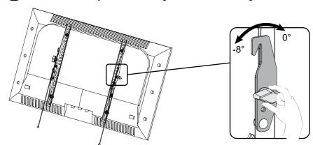
**Option:** To keep TV in vertical position, please use two M4 screws MA to insert the holes on two brackets respectively (as shown in below image).
