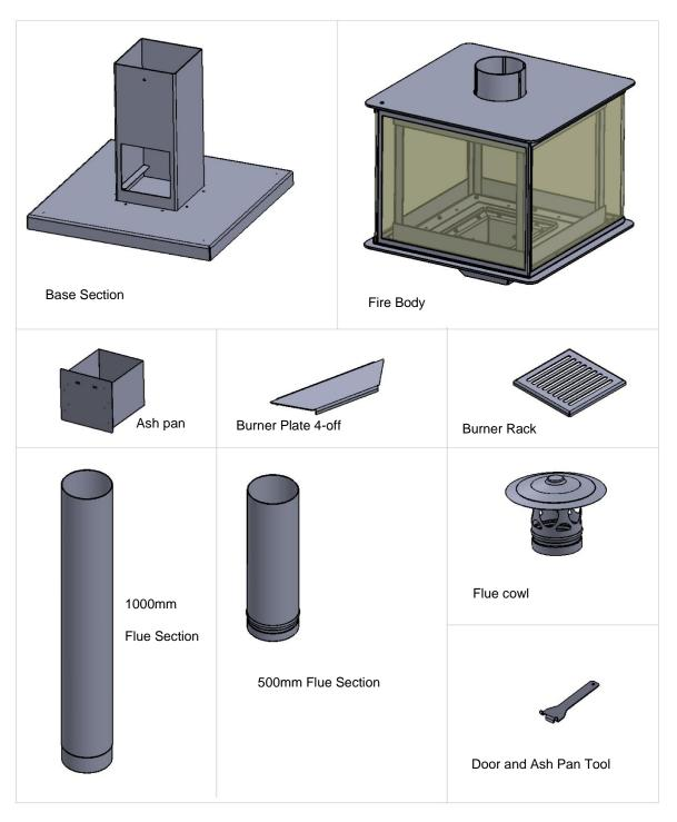
Dimensions of the cube w x d x h (600mm x 600mm x 960mm) plus height of the flue and cowl. **NOTE: The only tool required for assembly is a cross head screw driver.**
